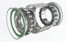
Personalized TDO bearing. 430222.XUDO Bore Ø 110 mm / Special Sealing material and design / Special bench end play to reduce mounting errors / Special Internal geometry to increase load capacities / Bering internal Grease capacity maximized to archive longer re-lub. Periods / Self-contained, pre-assembled and pre-lubricated / Reduces maintenance costs/ full reconditioning "ready" design.
