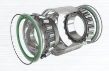
Personalized TDO bearing. 430222.XUDO Bore Ø 110 mm / Special Sealing material and design / Special bench end play to reduce mounting errors / Special Internal geometry to increase load capacities / Bering internal Grease capacity maximized to archive longer re-lub. Periods / Self-contained, pre-assembled and pre-lubricated / Reduces maintenance costs/ full reconditioning 'ready' design.
