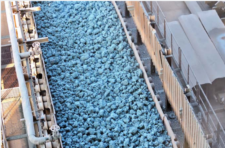
Figure 2-11. Apron conveyor carrying hot ore in a mining plant
