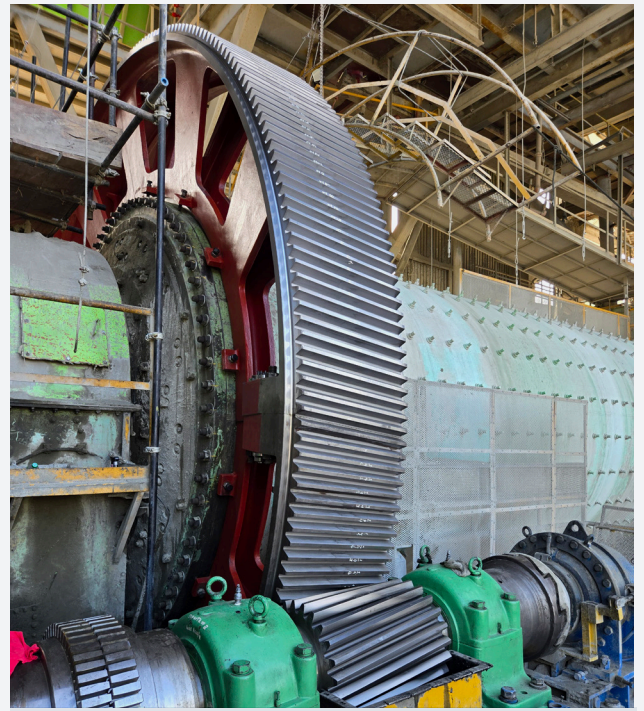
The image shows the girth gear, pinion shaft, and coupling manufactured by ABS and installed in the ball mill during the system alignment phase.
